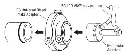
Install BG Injector Atomizer into BG Universal Diesel Intake Adaptor
