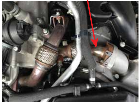
EGR cooler outlet pipe with EGR temperature sensor
