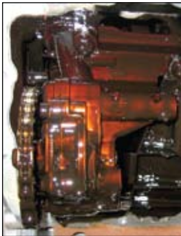
Sludge buildup in Volkswagen/Audi engine
